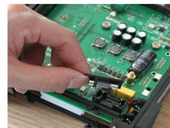
Figure 4 Remove the cover of fuse,
