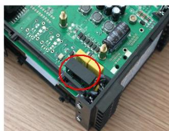
Figure 3 The black rectangular component is fuse
