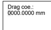
After setting Drag Coefficient, press SET key to Expansibility Submenu press Right key to shift cursor on Cursor position, and then press Up/Down key to change this value.
