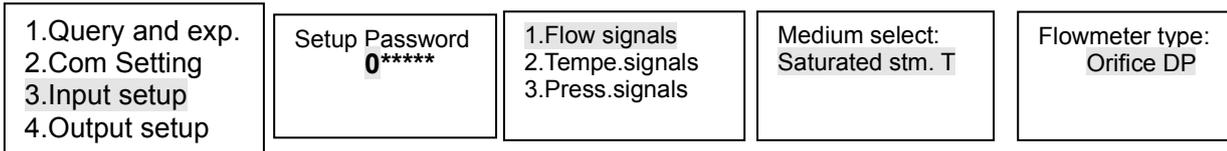
There are nine parameters in Orifice DP: Signal type, Pipe diameter, Hole diameter, Expansibility, Flow Coefficient, DP unit, DP low scale, DP high scale and Cut-off current.
