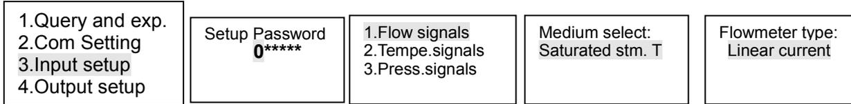
After the flowmeter type is set, Press the menu button to enter the current and the corresponding range setting.
