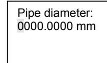
After setting Pipe Diameter, press SET key to Drag Coefficient Submenu, press Right key to shift cursor on Cursor position, and then press Up/Down key to change this value.
