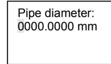
After setting Pipe Diameter, press SET key to Bend Radius Submenu, press Right key to shift cursor on Cursor position, and then press Up/Down key to change this value.
