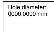
After setting Hole diameter, press SET key to Expansibility Submenu, press Right key to shift cursor on Cursor position, and then press Up/Down key to change this value.
