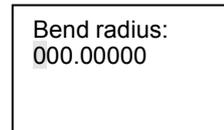
After setting Bend Radius, press SET key to Expansibility Submenu press Right key to shift cursor on Cursor position, and then press Up/Down key to change this value.
