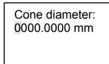
After setting Cone Diameter, press SET key to Expansibility Submenu press Right key to shift cursor on Cursor position, and then press Up/Down key to change this value.
