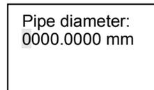
After setting Pipe Diameter, press SET key to Cone Diameter Submenu, press Right key to shift cursor on Cursor position, and then press Up/Down key to change this value.
