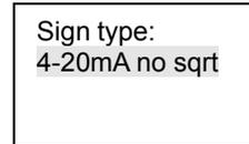
After setting Signal type, press SET key to Pipe Diameter Submenu, press Right key to shift cursor on Cursor position, and then press Up/Down key to change this value.
