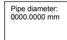
After setting Pipe Diameter, press SET key to Hole Diameter Submenu, press Right key to shift cursor on Cursor position, and then press Up/Down key to change this value.
