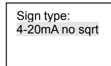
After setting Signal type, press SET key to Pipe Diameter Submenu, press Right key to shift cursor on Cursor position, and then press Up/Down key to change this value.
