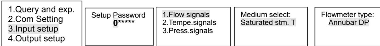
There are nine parameters in Annubar DP: Signal type, Pipe diameter, Drag coefficient, Expansibility, Flow coefficient, DP unit, DP low scale, DP high scale and Cut-off current.
