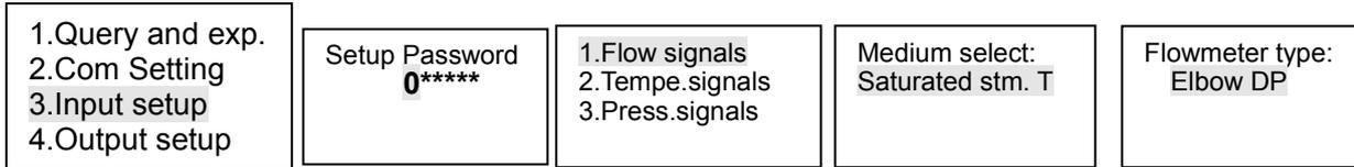
There are nine parameters in Elbow DP: Signal type, Pipe diameter, Bend radius, Expansibility, Flow coefficient, DP unit, DP low scale, DP high scale and Cut-off current.
